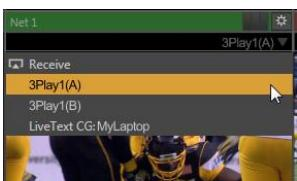
3Play's *Output A* and *Output B* are available as *Switcher* sources to TriCaster. They appear in the source selector menu for TriCaster's *network* inputs as "3Play(A)" and "3Play(B)," where "3Play" is the name for the system.
